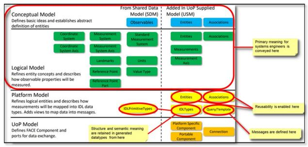
Figure 3: UDDL Data Architecture Traceability to Entity Model.
