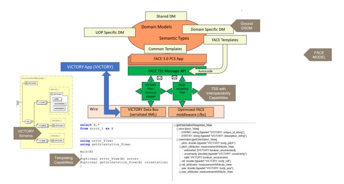
Figure 6: FACE-VICTORY Adapter Demonstration Architecture
